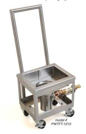
Section 701.7 of the International Plumbina Code mandates that water entering a drainage system cannot exceed 140°F, which could cause problems with PVC pipes and other safety and environmental issues. The Cool Trough™ is designed to activate the temperature sensor at 130°F and turn off the mixing valve at 120°F, thus using water only when required.
